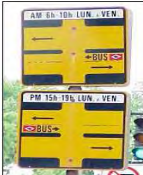
Figure 2-27 Bus lanes are frequently in effect only during the peak hours in the peak direction
